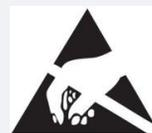
ESD Protection: Strictly adhere to ESD precautions to prevent electrostatic damage.
