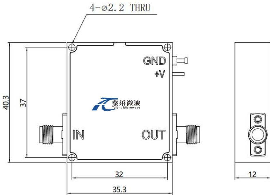
\*\*\*Heat Sink Required During Operation
