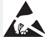
ESD Protection: Strictly adhere to ESD precautions to prevent electrostatic damage.
