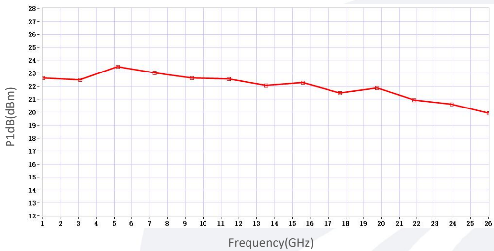
P1dB vs Frequency
